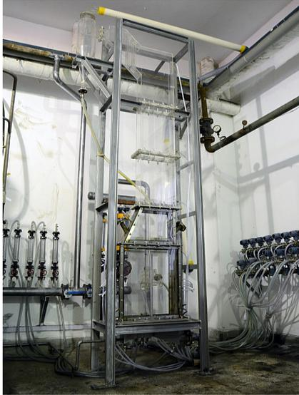
**Figure 5.** Cold Flow Model Constructed of Plexiglas®, ¼ Scale of Hot Pilot Plant, Used to Validate System Hydrodynamics
